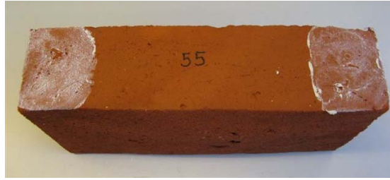
Figure 5. Brick after use of an oxide coated titanium anode. No visible discoloring from the anode. The white areas are kaolin clay and can be minimized by use of e.g. porous paper between the brick and the kaolin clay.
