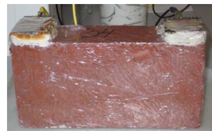
Figure 2. Laboratory setup where the poultice with electrodes is placed on the long, narrow side of the brick.
