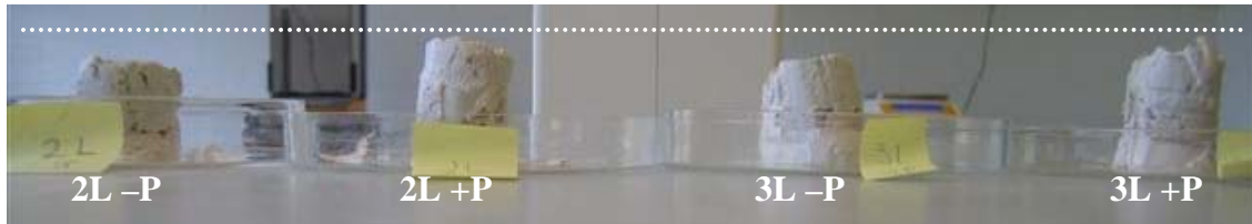
Figure 3. Visible variation in the height after ended tests (11 days). The highest volume decrease was seen left (2L-P) and the lowest right (3L+P). The dotted white line indicates the initial height, however minor visual changes happened during the plastic tubes were removed.
