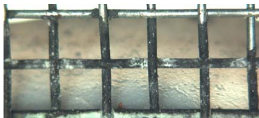
Figure 5. Decomposition of the anode mesh made of stainless steel. The original metallic gray color is during the decomposition changed to black and later green and the metal mesh will subsequently get so deteriorated that it breaks. Stainless steel is surface coated iron.
