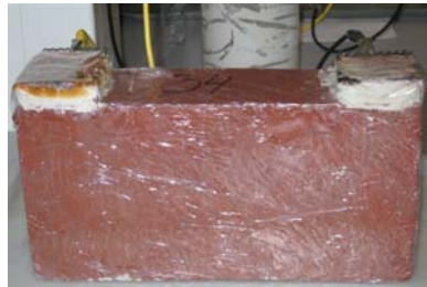
Figure 4. Laboratory setup where the electrodes (and poultices) both are placed on the bricks long, narrow side.
