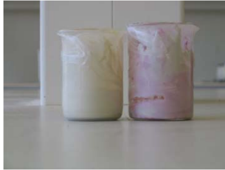
Figure 1. The acid-base color indicator change in kaolin clay from beige (left) at pH above 6.3 to red (right) at pH below 6.3.
