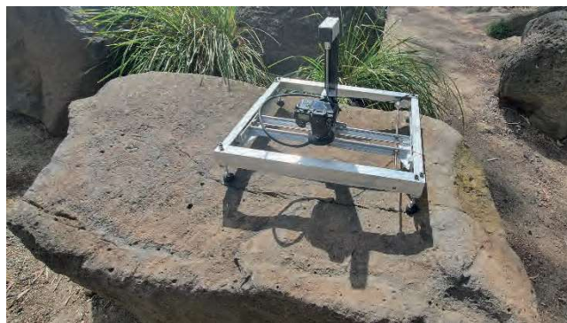
Figure 2: The microscope on camera positioned above the surface in the motorized frame. Levelling feet maintain a minimal scanning height range across the plane.
