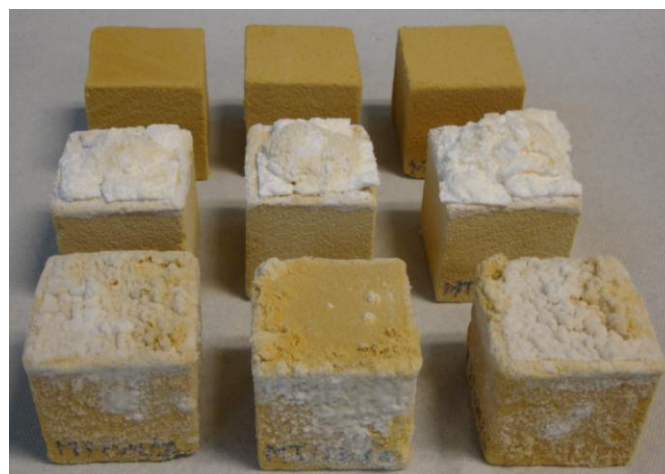
Figure 6. Maastrichter samples after 10 days at 20°C and 85% RH, previously contaminated with NaNO 3 (up), Na 2 SO 4 (middle) and an equimolar mixture of Na 2 SO 4 and NaNO 3 mixture (bottom).
