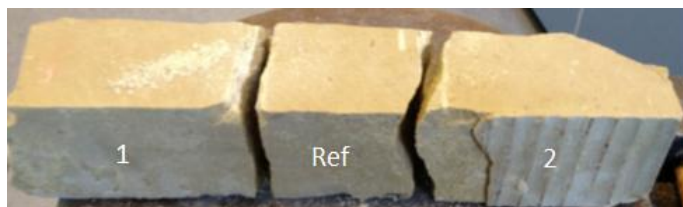
Figure 2: Segmentation of a stone piece into a reference segment (Ref) and segment 1 and 2 for desalination experiments.
