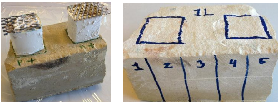
Figure 4: Experiment 1. (a) Placement of the electrode units and (b) Segmentation of the stone segment into slices at the end of the experiment
