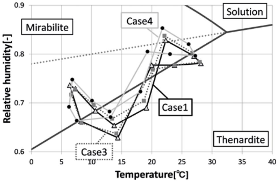
Figure 12: Phase diagrams for Case 1, Case 3 and Case 4
