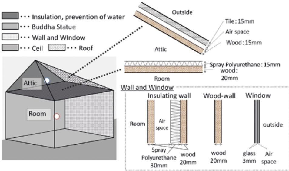
Figure 6: Model for analysing the room environment
