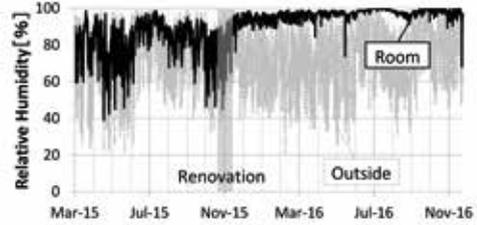
Figure 4: Variation of the measured relative humidity inside and outside the shelter
