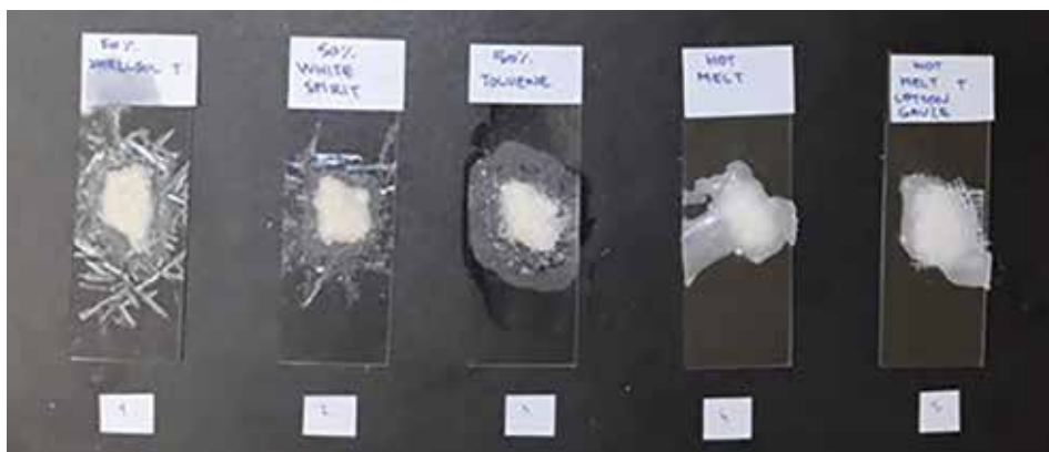
Figure 1: Glass slides with Seget powder and different types of application of CDD (from left to right: 50% solution of CDD in Shellsol T; 50 % solution of CDD in white spirit; 50 % solution of CDD in toluene; hot melted CDD; hot melted CDD with cotton gauze)
