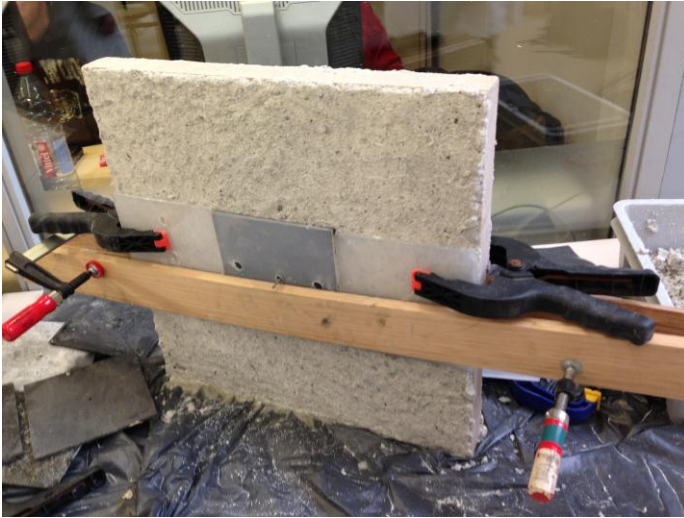
Figure 2: The electrodes, applied in the middle of the opposite sides of limestone plates of 45x45x4 cm, are kept in place using a wooden panel on both sides and positioned by means of screws. A plastic plate applied between the wooden panel and the contact material serves as protection for the contact material underneath it.
