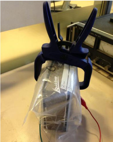
Figure 1: Setup for the limestone plates of 15x15x4 cm
