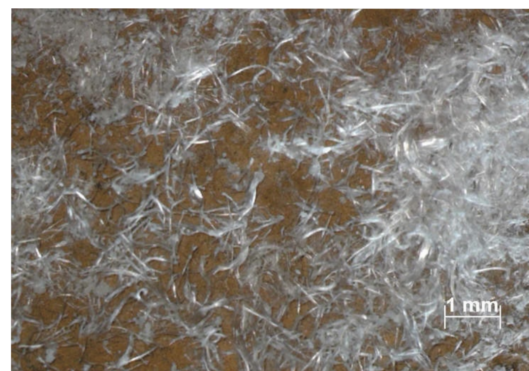
The efflorescence occurred on calcium containing objects stored in oak wooden cabinets for a long period of time.
