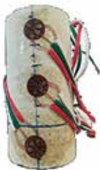
Figure 2: Sample pollution process (a), sample of tuffeau with strain gage rosettes (b)
