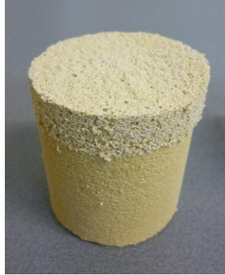
Figure 2: Specimen with a surface layer presenting insufficient cohesion, obtained by re-aggregating stone grains used for testing consolidant products
