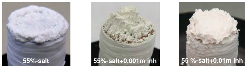
Figure 4.14: Pictures of the efflorescence formed at the end of drying experiment in case of salt saturated brick with and without inhibitor dried at 55% RH. A comparable amount of efflorescence was formed in both cases, i.e., with and without inhibitor.
