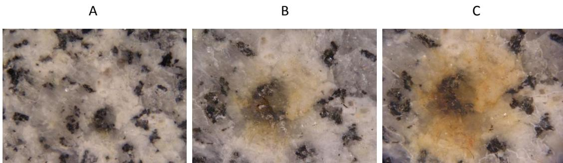
Figure 4. Photos from the same sample surface of the CE granite (x10 magnification): A) Before the SCA test; B) After 75 cycles; C) After 150 cycles.
