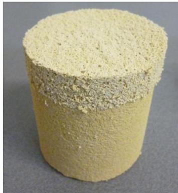
**Figure 2:** Specimen of Maastricht limestone with re-aggregated layer on top
