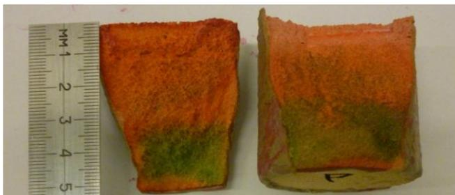
**Figure 5:** Penetration depth of ethyl silicate in a specimen with re-aggregated top layer (the pink-orange colour indicates the presence of the treatment)
