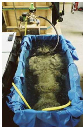
Figure 1. Sandstone vase in water bath for desalination in routine procedure.
