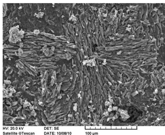
Figure 8. Rosette- like gypsum crystals cover the surface of the sample (SEM image).
