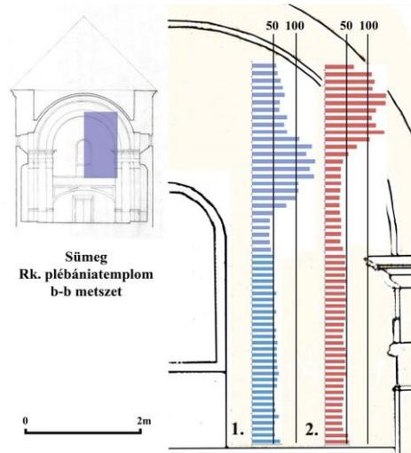
Figure 5. Cross section of the church (left) with two moisture content measurements (right) showing increasing moisture content along vertical profiles of the choir showing the downward migration of moisture from the ceiling (length of horizontal bars are proportional with the moisture content).
