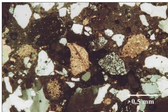
Figure 6. Fine angular grains of various mineral composition (quartz, calcite) in the upper plaster layer embedded in calcareous matrix (transmitted light microscopic image, crossed polars).
