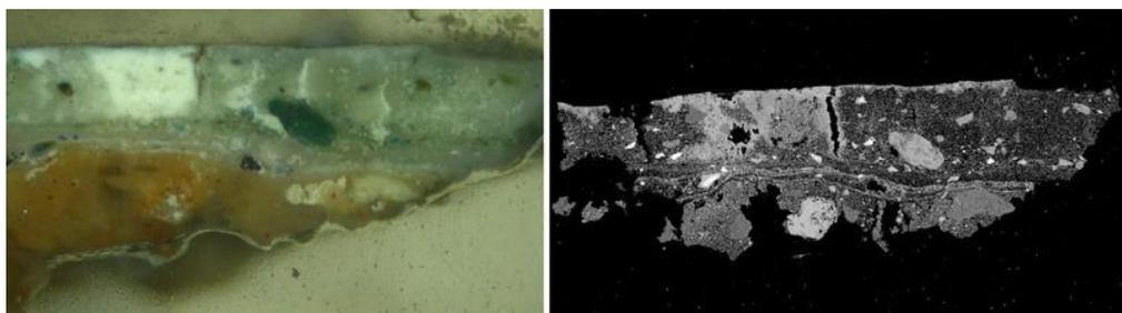
Figure 7. Cross section of the original painted layers, showing a light blue underpaint with smalt, and a greenish layer with green earth and lime. (left: reflected light, right: SEM –BSE).
