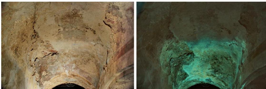
Figure 3. Normal light (left) and UV luminescence (right) image depicting the badly damaged zone (bright zones on the UV image) of the fresco, in the the NW Choir of the church.
