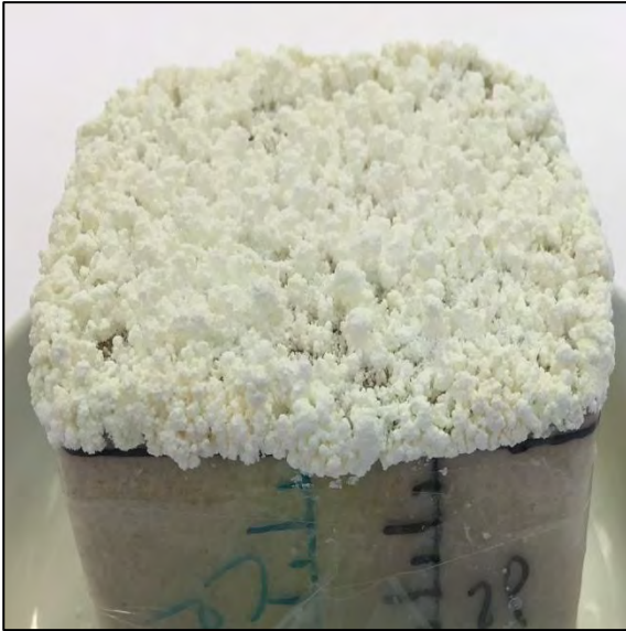
Fig. 6.15: Efflorescences formed at the end of drying process on sample 11-50 salinated with salt mixture and treated with 0.1% inhibitor solution.
