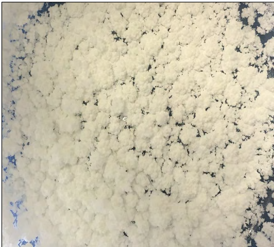
Fig. 6.10: Dendritic crystal system of NaCl and KCl in the presence of inhibitor
