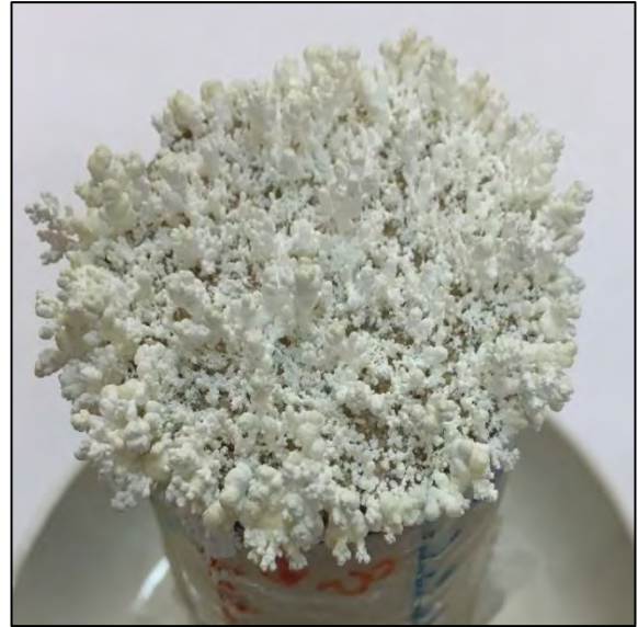
Fig. 6.16: Efflorescences formed at the end of drying process on sample 9-1 salinated with salt mixture and treated with 1% inhibitor solution.
