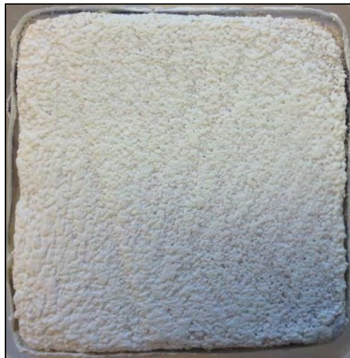
Fig. 5.22: Salt crust formed at the end of treatment process
