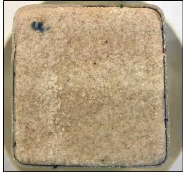
Fig. 6.28: Salt crust and efflorescence formed at the end of drying process on sample 11-7 salinated with salt mixture and treated with 0% inhibitor solution.
