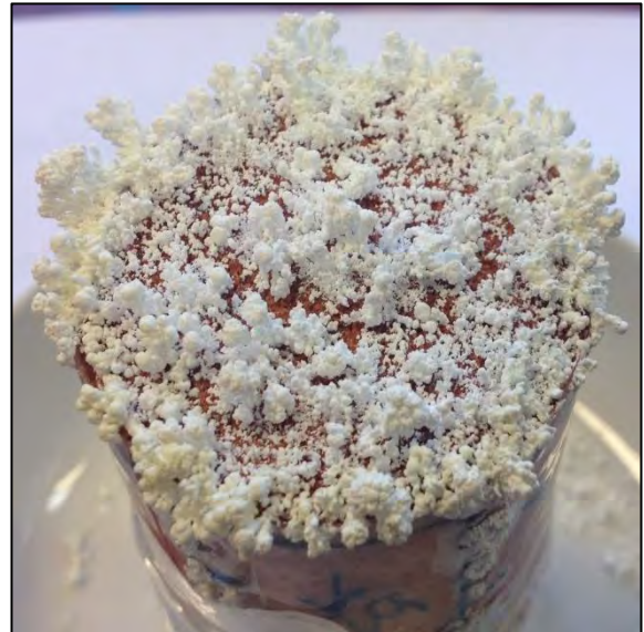
Fig. 6.18: Efflorescences formed at the end of drying process on sample 2-4 salinated with saturated solution of NaCl and treated with 1% inhibitor solution.
