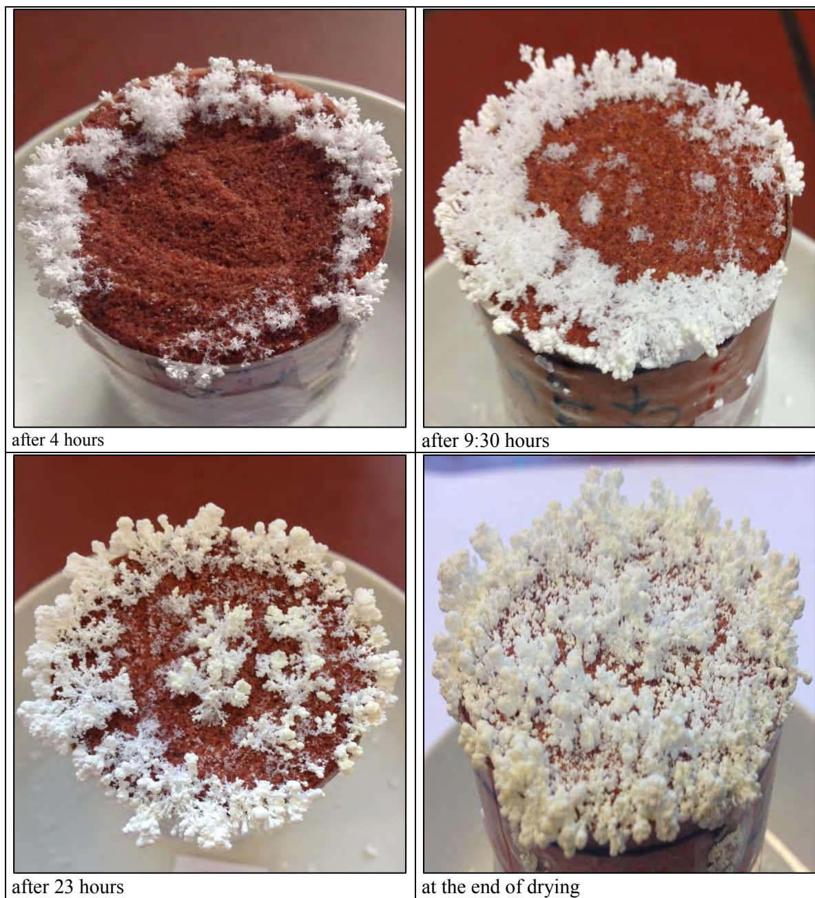
Fig. A.7.1: Formation of efflorescences in the course of drying, sample 2-4 salinated with saturation solution of NaCl, treated with 1% inhibitor solution
