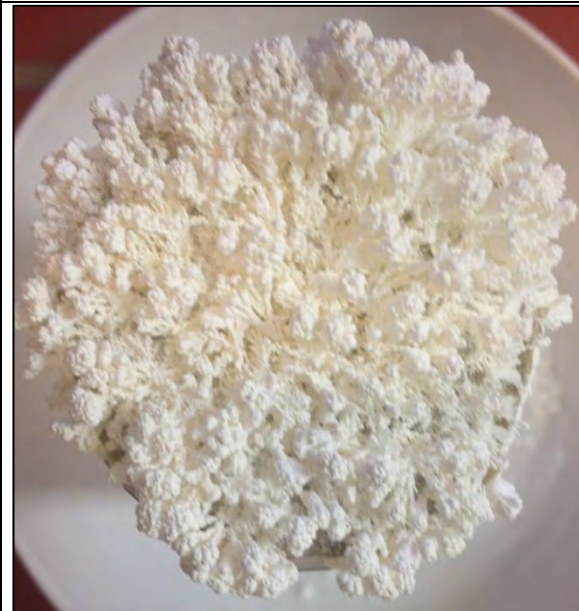
Fig. A.7.3: Formation of efflorescences in the course of drying, sample 3-4 salinated with saturation solution of NaCl, treated with 2% inhibitor solution
