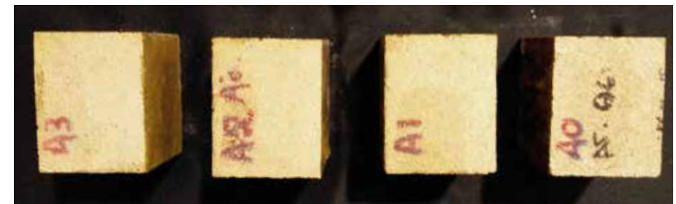
Figure 3: Physical appearance of the stone surfaces before/after each treatment. A0: Untreated stone, A1: Oleic acid treated stone, A2: Sodium oleate treated stone, A3: Calcium oleate treated stone
