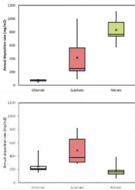
Figure 5: Annual deposition of salts on passive samplers from historic buildings situated at traffic-rich urban main roads. Left: Results for SAM-samplers. Right: Results for stone samples.
