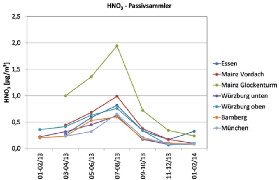
Figure 6: Results from passive sampling of HNO<sub>3</sub> at various facades. Data by courtesy of the Swedish Corrosion Institute, from <sup>12</sup>
