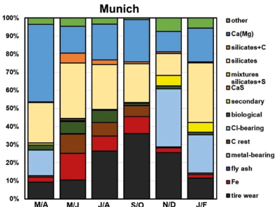
Figure 3: Variation of the composition of deposited particles  $> 3 \mu\text{m}$  at Munich (relative surface coverage). Letters on x-axis indicate bi-monthly sampling. From <sup>11</sup>
