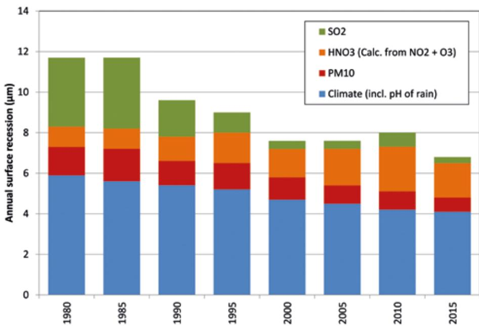
Figure 2: Calculated recession rates of Portland limestone under environmental conditions of the Karlsplatz at Munich during the last 35 years. Modified from<sup>9</sup>
