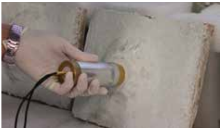
Figure 2: SUSI® measurements on a replica after 48 hours from the injection
