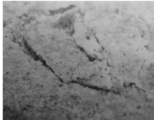
Figure 5.15 (left) Bulging and scaling of the outer layer of a brick specimen after 3 drying cycles at 21.5^{\circ}\text{C} , 50% RH and airflow
