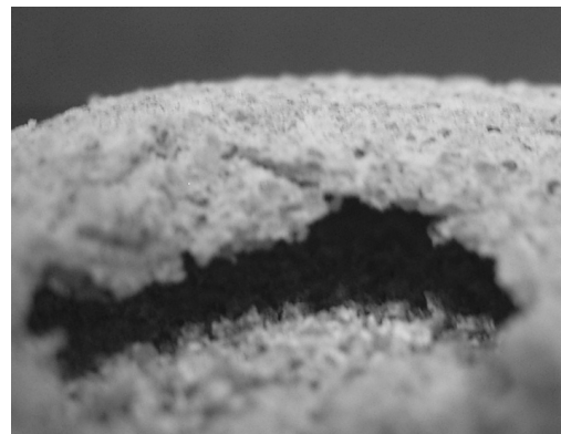
Figure 5.17 (left) Bulging of the outer layer of a lime-cement mortar specimen after 2 drying cycles at 60^{\circ}\text{C} / 0% RH
