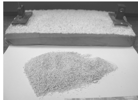
Figure 6.5a (left) Sanding of the outer layer of the mortar in the presence of NaCl after 6 RH cycles Fig.6.5b (right) Material brushed from the surface of the mortar after 6 RH cycles
