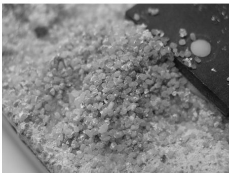
Figure 6.5a (left) Sanding of the outer layer of the mortar in the presence of NaCl after 6 RH cycles Fig.6.5b (right) Material brushed from the surface of the mortar after 6 RH cycles
