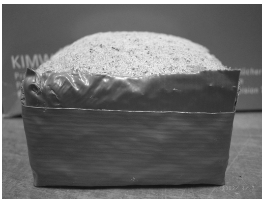
Figure 5.17 (left) Bulging of the outer layer of a lime-cement mortar specimen after 2 drying cycles at 60^{\circ}\text{C} / 0% RH
