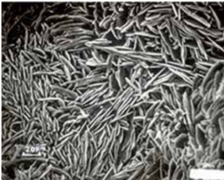
Figure 3: SEM photomicrographs of the gypsum efflorescence on brick, left (see Fig.2 left), and the framboidal growths resulting from air pollution on limestone of the Cowper Hewitt Museum, right.
